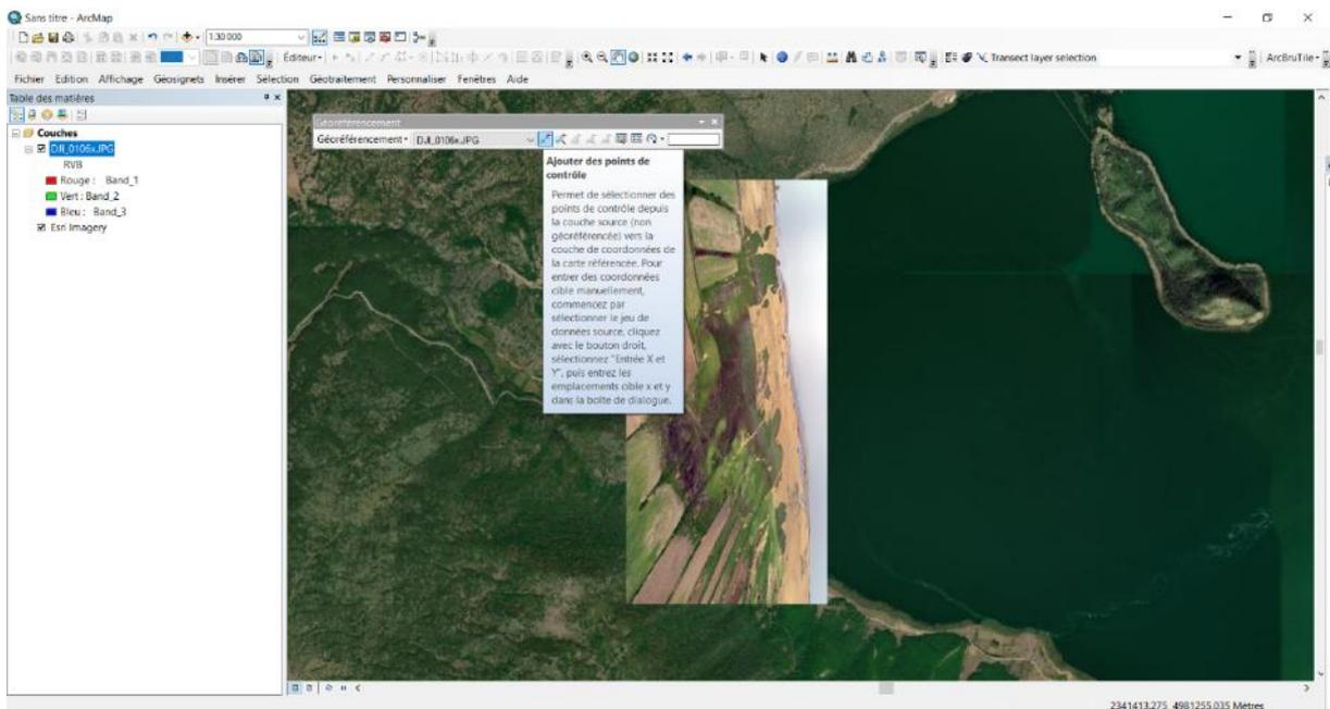
First, click on the jpg file on an identifiable landmark. It displays a green cross.
