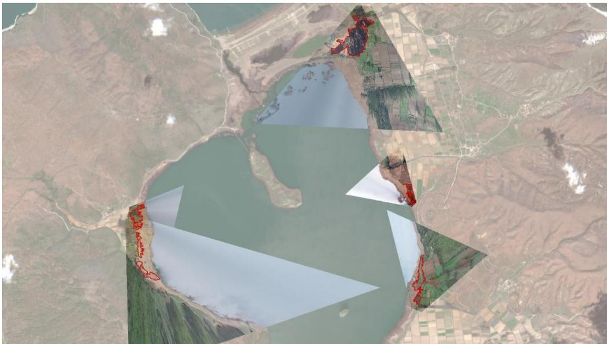
To be even more accurate, you can adjust a correction when you draw your polygons to delineate the part hidden by the height of the reed, according to the position of the drone's point of view:
